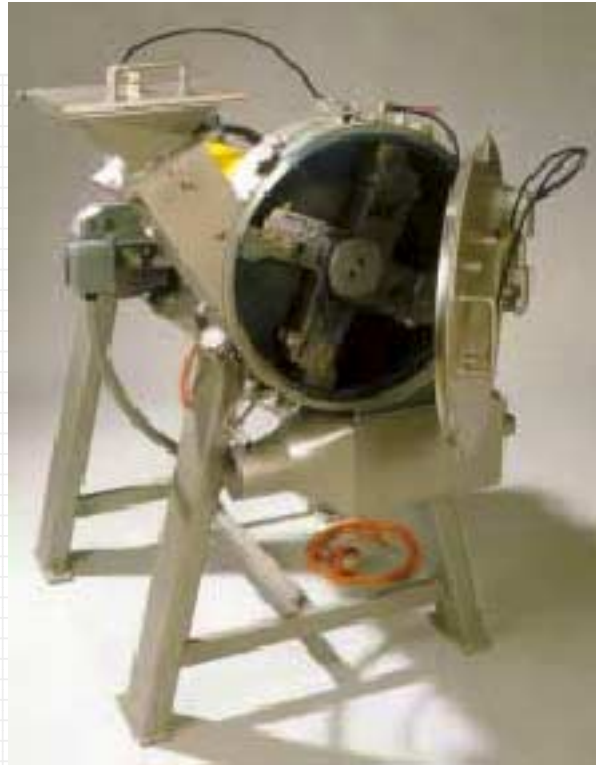
Labtech Essa 450 mm dia. Hammer Mill (without dust hoods)
