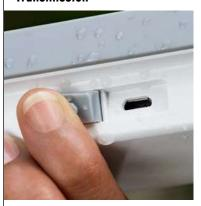
Thanks to its IP67 protection and drop test resistance, the new Seven2Go portables are able to withstand harsh and demanding environments. The weatherproof USB connector ensures data can be transferred safely even after the meter has been exposed to heaps of water.
