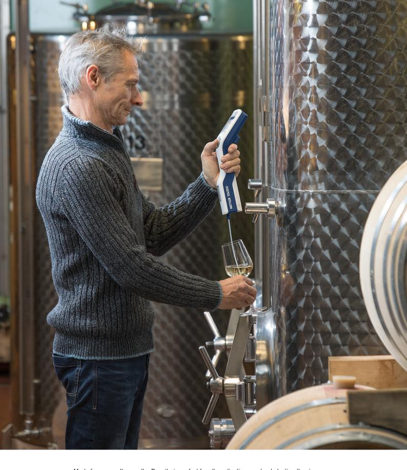
Made for use on-the-go, the Densito is perfect for all applications: not only testing the ripeness or fermentation of grapes, but also the quality of incoming goods or final products. Measure density, specific gravity, Brix, and many more using built-in calculations on the instrument. Its unique design allows for one-handed operation, leaving your second hand free to aid you in the sampling process.
