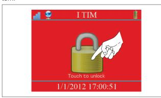
To unlock the dialler, tap the padlock in the centre of the screen and enter the administrator password (default setting "12345") using the touch keypad. Then tap confirm in the bottom right corner.
