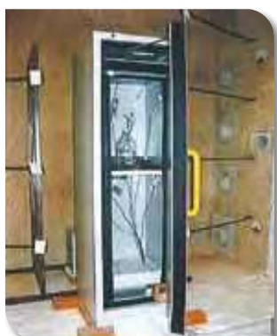
CHEMISAFE cabinet series FIRE MY11 BEFORE fire resistance test.
